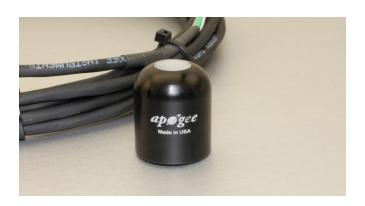
The SP-series silicon cell pyranometers are available in self-powered voltage, amplified voltage, and current output options. They are calibrated to measure total shortwave radiation. This cosine-corrected sensor is designed to maintain its accuracy when radiation comes from low zenith angles. This accuracy is shown in the graph below. The SP-110 closely matches the Kipp & Zonen CM21.
